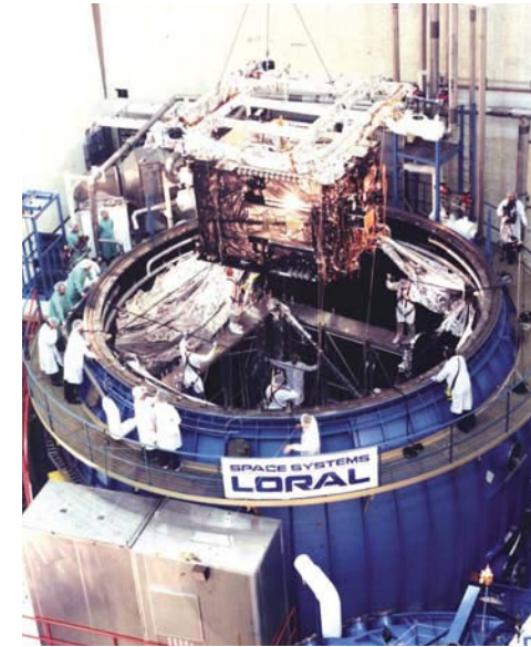
Optus-C1 was lowered into the thermal vacuum chamber at Space Systems/Loral in 2002. Now it provides communications coverage for Australia, New Zealand, and Asia, as well as a hosted payload for the Australian Defence Forces.
